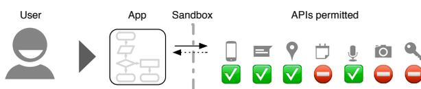
**Figure 1: Sandbox mining in a nutshell.** The mining phase automatically generates tests for an application, monitoring the accessed APIs and resources. These make up the *sandbox* for the app, which later prohibits access to resources not accessed during testing [2].
